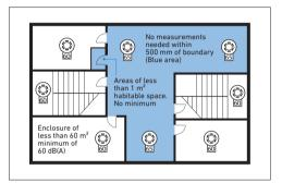
The minimum sound level should be 65 dB(A) or 5 dB(A) above a background noise which is louder than 60 dB(A) (if lasting more than 30 seconds) and at a frequency of between 500 Hz and 1000 Hz. The maximum sound level should not be greater than 120 dB(A) at any normally accessible point. May be reduced to 60 dB(A) in stairways, enclosures up to 60 m² and specific points of limited extent. If using fire alarm as as lockdown alarm this must be a distinctly different tone to that of the fire alarm.
